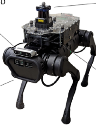
Fig 2: The autonomous robotic dog (from Unitree) equipped with the efficient multisensor intelligent backpack, designed by ETH for low-latency multi-sensor fusion perception and embedded control.
