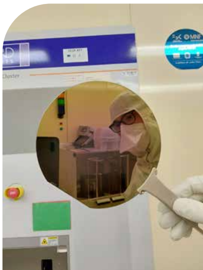
Amorphous Silicon Carbide layer deposited on silicon wafer by FBK-SD.
