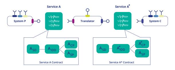
Information interoperability between two service providers can be addressed by means of translators. The design of such translators for the payload information is currently necessary to provide for every situation where interoperability is requested.
