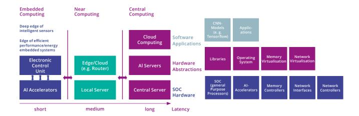
The continuum of computing and relations between the elements constituting an embedded AI system (figure from Gerd Teepe)
