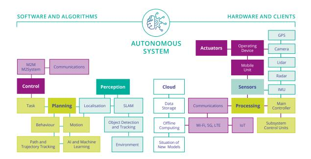
A generalised overview of autonomous system (AS) technologies and functionalities. Adapted from Pendleton, S.D., Andersen, A., Du, X., Shen, X., Meghjani, M., Eng, Y.H., Rus, D., Ang, M.H.Jr. (2017). "Perception, Planning, Control, and Coordination for Autonomous Vehicles. Machines", 2017.
