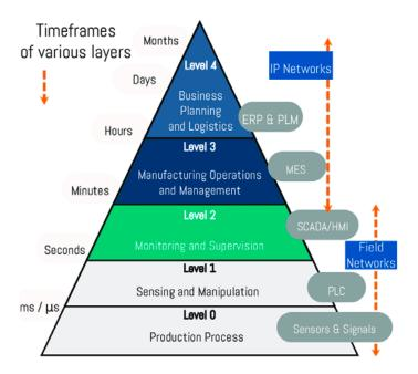
$ISA95\ Hierarchy\ Model\ with\ building\ blocks\ of\ Autonomous\ Systems\ according\ to\ the\ 5\ levels\ of\ the\ conventional\ automation\ pyramid ^{152}$
