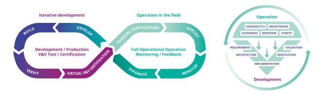
Simplified examples for continuous development processes (DevOps processes), Such processes are essential for building future ECS-based systems and products since they enable data collected during the operation phase to be used in iterative (continuous) development for updates of existing products.
