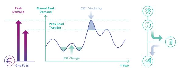
Visualization of an algorithm-controlled energy management system to shave peak loads. An energy storage system predicts load peaks and charges/discharges a battery accordingly. Source: EDF Renewables.
