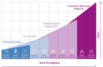
Example of architecture of a modern SoC (from Paolo Azzoni, see also Chapter 1.3) / Arm's Cortex-M55 and Ethos-U55 Tandem. Provide processing power for gesture recognition, biometrics, and speech recognition applications (Source: Arm).
