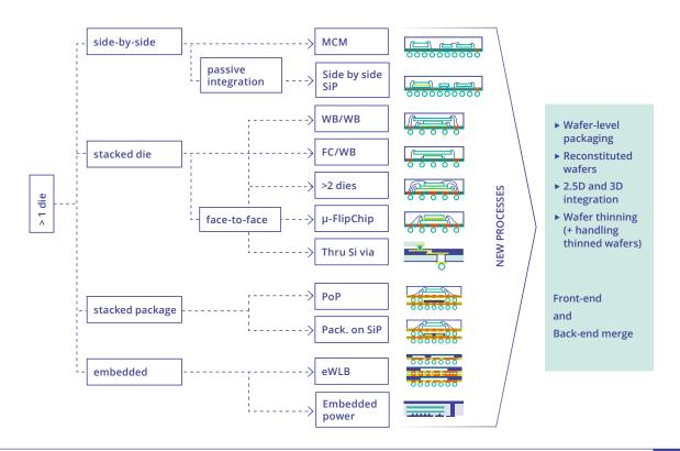
System in a package (SiP) examples. With merging of front-end and back-end, almost unlimited possibilities enabled (Source: Andreas Grassmann – Infineon – 3D Systems Summit)
