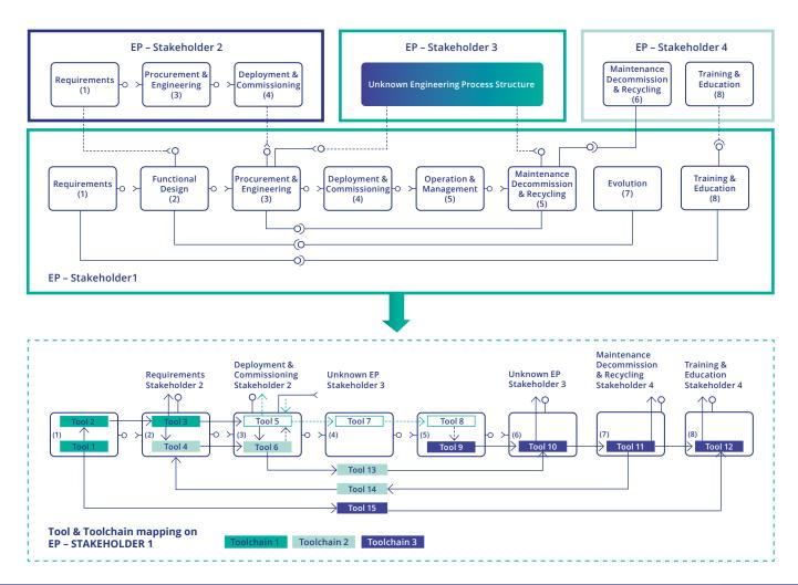
Example of conceptual service-oriented view on the integration of multiple service-based engineering processes (EP) from different stakeholders, including the engineering process mapping with integrated toolchains and tools $^{24}$
